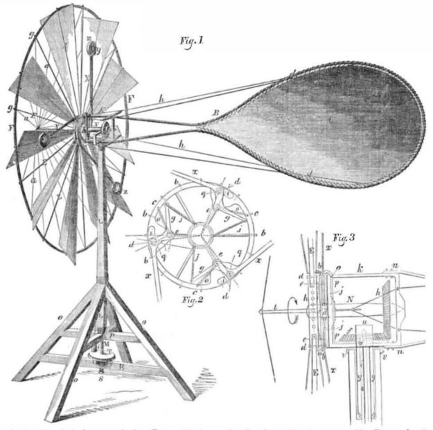
by the regulation wheel. In strong and sudden gusts of wind, the regulator is not dependent upon the velocity of the mill for its operation, but upon the inertia of the weights. the wheel will instantaneously start, but the so that the sails are as instantaneously, or simultaneously, turned edgewise to the wind. Otherwise, before the necessary velocity for operating the regulator could be obtained, the mill might sustain injury.
