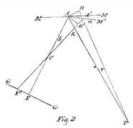
Let A M, A M, fig. 2, be the two mirrors, and A the hinge. Then the camera being supthe line of its axis, and also the direction of tion of one of the mirrors after its displacearrangement of lenses, the image of P will be formed at F', instead of at F, by means of the the glass screen, will of course be perpendicular to the axis, A F.
