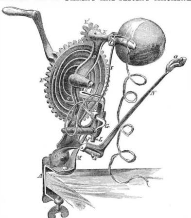
Machine for Paring and Slicing Apples.
