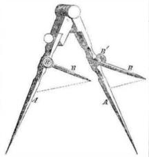
Proportional Dividers are generally large, costly, and somewhat clumsy. But the invention here illustrated consists of a simple and inexpensive attachment to the common dividers. A A are the long legs to which the short legs, B, are attached, as shown. This constitutes the chief feature of the improvement. The short legs are fastened by the adjusting screws, B'.
