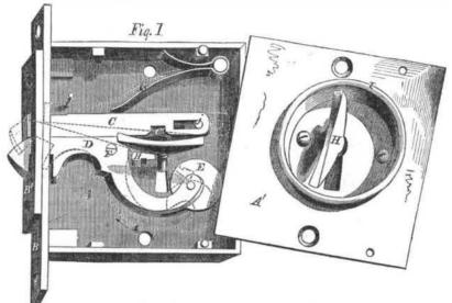
The acompanying engravings are illustra- i shown in fig. 1, the latch, D, is fastened down, tive of the improved Latching Lock patented and holds firmly in catch-piece, B'. Turn in this country by Mr. Edmund Field, of Greenwich, Ct., July 3rd, 1855, and in Europe April, 1855.
