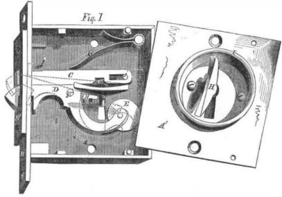
The acompanying engravings are illustra- ishown in fig. 1, the latch, D, is fastened down, tive of the improved Latching Lock patented and holds firmly in catch-piece, B'. Turn in this country by Mr. Edmund Field, of Greenwich, Ct., July 3rd, 1855, and in Europe April,
