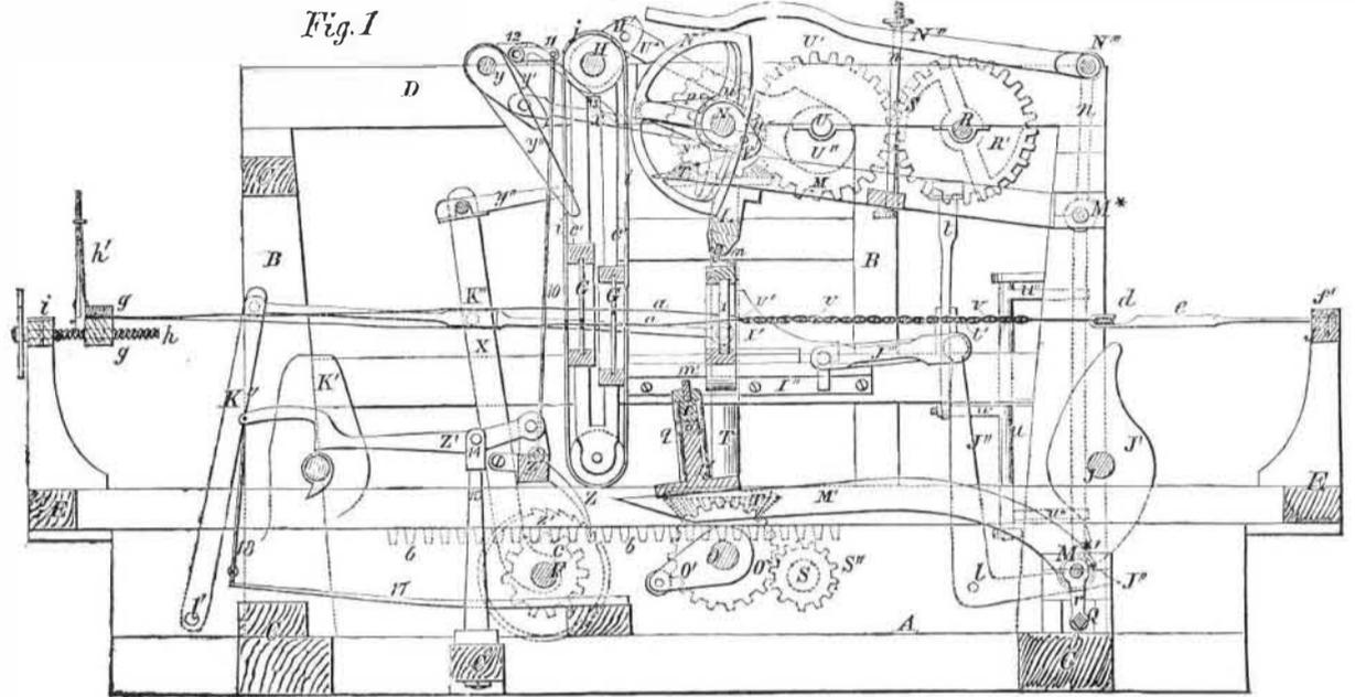
suitable mechanism, the clamps, g g, admitting of this drawing forward, as they only grasp it just tight enough to keep the wires properly extended and straight. The work is then again secured, the front part being secured this time by clamping it directly between the clamps, f f, the hooks, e e, being no longer necessary, and the rear part being secured by the tongs, h', as before. When all is secure, the pawls, Z, are thrown out of gear,
