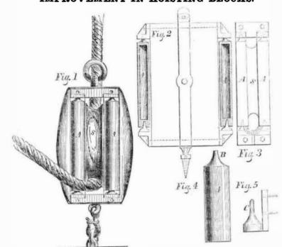
on ship board or shore, it is frequently necessary to change the bend of the rope, so that while one portion moves, for example, perpendicularly, the other part moves horizontally. Such a change of bend is indicated by the rope in fig. 1.
