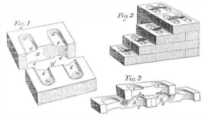
lately obtained a patent for an improvement in the form of bricks, which promises to be of If the usual care is taken in sorting out from some importance. The accompanying engravings are illustrative of the invention.
