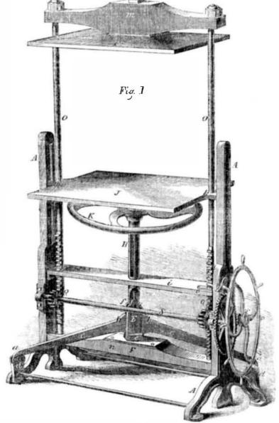
described, by means of the side wheel, T, the wheel, K, receives a few turns to block up the press, which brings the levers again into effective operation. When the operation is completed, the movable frame is raised sufficient to relieve the nut wheel, K, which may be turned back, the press let down, and the article removed.
