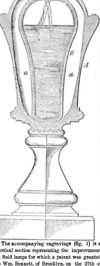
vertical section representing the improvement in fluid lamps for which a patent was granted to Wm. Bennett, of Brooklyn, on the 27th of of Nov. last, and fig. 2 is a vertical section of the patent safety tube-for spirit fluid lamps Washington st., this city.
