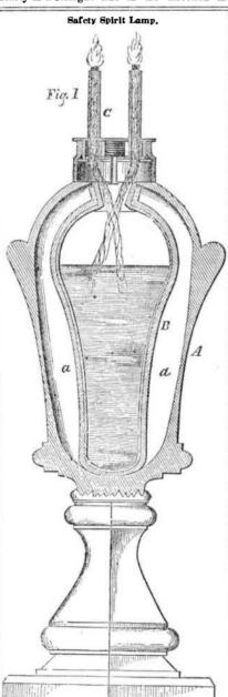
The accompanying engravings (fig. 1) is a vertical section representing the improvement in fluid lamps for which a patent was granted to Wm. Bennett, of Brooklyn, on the 27th of of Nov. last, and fig. 2 is a vertical section of the patent safety tube-for spirit fluid lamps the patent having been assigned to the B is the collar which is secured on the lamp. Union India Rubber Lamp Co., office No. 284 A is the cap which screws into the collar. D Washington st., this city.
