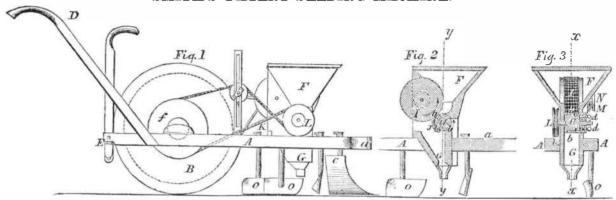
the drill, and is covered by the shares, O O double share, C, and the wheel, B, passes over and presses the earth on the seed.
