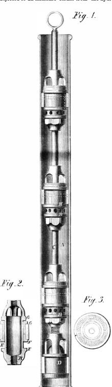
static pressure due to the long column of oil that has to be lifted at each stroke. This pressure is very great, and not only causes the packing to wear leaky in a short time, but it also endangers the safety of the pump barrel itself, which not unfrequently bursts from the severe strain of resisting the movement of oxydation.'
