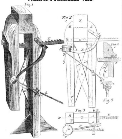
The accompanying engravings represent the | shall be tightened by pressure upon a simple improvement in Parallel Vises, for which a pat- lever, without the agency of screw power in ent was granted to Jasper Johnson, of Geneseo, any form; a gathering pawl which constitutes
