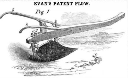
The accompanying figures illustrate the im- | ble at pleasure by means of convenient screws; provements in plows for which a patent was also to elevate and lower the beam by slide, granted to L. G. Evans, of Spring Hill, Ala., wedge, or other similar device. on the 19th of June last. Although the plow
