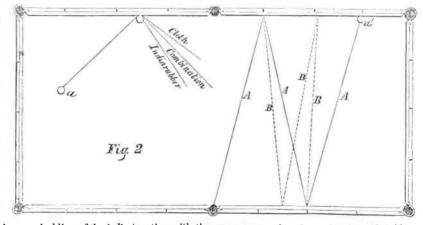
in or embedding of the ball, together with the objections referred to in the old table are the angle produced by the rebound, being improvements are introduced. The "combinaacute, and so much at variance with correct angles. Fig. 5 is a sectional view, representing the new "combination" cushion, in which
