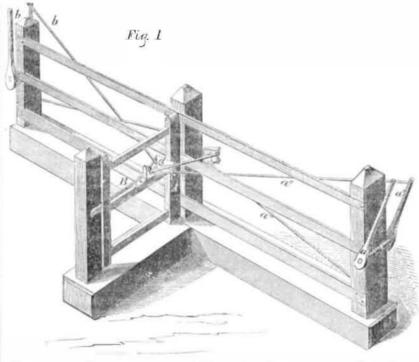
Fig. 1 of the accompanying engraving is a | lever, a, as shown in fig. 1. The cord, a2, is perspective view, and fig. 2 is a plan view of a attached by one end to the top of lever a', and method of operating gates for farms, for which by the other end at c, fig. 2, to the semi-cylina patent was granted to John K. Weber, of drical segment, d, which is firmly fixed to the
