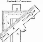
The accompanying figure is a view of an instrument bearing the above name, designed for a square, scale, level, and bevel-very dipersede water saw mills, which are usually versified uses—for which a patent was granted placed in unhealthy localities, especially in to Josiah Shanklin, on the 4th of October, last
