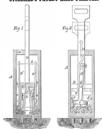
The accompanying engravings represent the | part of the smaller case, B, there are attached of the gate or slide, F, there is attached a rod, improvements in hand Corn Planters, for which two springs, b b, at opposite sides. The lower a patent was granted to Oren Stoddard, of ends of these springs are attached to bars, cc, Busti, Chatauque Co., N. Y., on the 26th of to which bars perforated plates or dropping The two figures are vertical sections (taken
