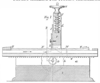
back of the gate or slide, F, will strike the in- position by turning the shaft, E, in the reverse clined wedges or planes, M M, and the gate or direction, and the stop, g, on the opposite end slide, F, will be forced upward beyond the of the carriage will strike the inclined planes reach of the patterns, L L. The finished strips or wedges and throw them out from underare then removed and others secured to the neath the plate, J, thereby allowing the spring, addressed to the patentee.
