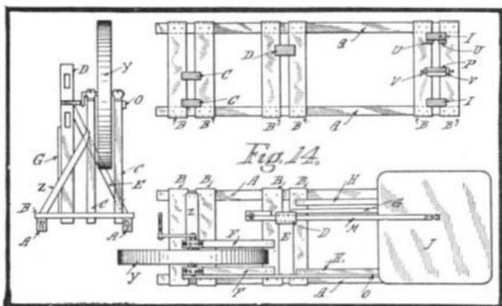
The hardwood pulley R is 6 inches diameter and 5 inches face. It is secured to the shaft in the manner shown in Fig. 11. A simple brake, made from a piece of 3-inch by 4-inch timber, shaped on one edge to fit the rim of the wheel, and operated by the foot, is shown in Fig. 11, it having been omitted in the general views. The connecting rod T is made from hardwood, 21 inches long, 18 inches center to center of
