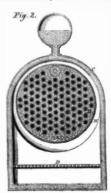
man-hole, F, and space, G, by which access may be had to the inside of the boiler. The operation of this boiler and the course of the flame and heat is shown by the arrows; from the furnace the caloric rises hrough the passages, H, and completely surrounds he internal cylinder, and passing through the small adise. Enervated, languid, emaciated as they are, in
