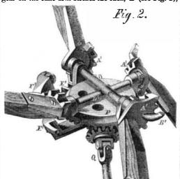
the rake is gradually elevated from the grain platform, and is carried round again (as at T, in Fig. 1) to the platform; the tongue, B', on the lower end of the gear, A, slides upon the guard, F', which sustains the rake while passing over the operator's head. The seat for the driver is shown at U.
