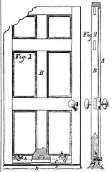
the bar, C, may be lowered by adjusting the set screws, d. which secure the bar in the groove, b, in the lower edge of the door. The heads of the set screws may be of any proper form so as to be rather ornamental than other-
