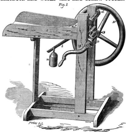
The accompanying engravings are views of | length of the cylinder, and parallel with it.an improvement in straw cutters for which a The knives are attached to the cylinder at oppatent was granted to Thomas C. Simonton, posite points on its periphery. and Loren J. Wicks, of Paterson, N. J., on the 10th of April last.
