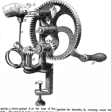
fork. The wheel, E, is then turned by the han- frame, and its knife bearing against the apple dle, F, and the apple rotates. The wheel, j. al-
