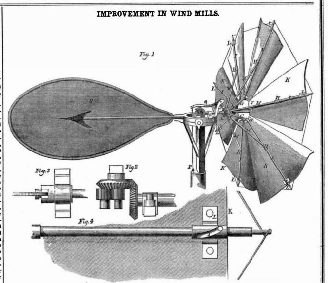
provement in Windmills, for which a patent It is allowed to slide on the shaft, C, to which the spring, F, by increasing the weight. was granted to Addison P. Brown, of Brat- it is secured by a key working in a spline or tleboro', Vt., on the 3rd, of this month.
