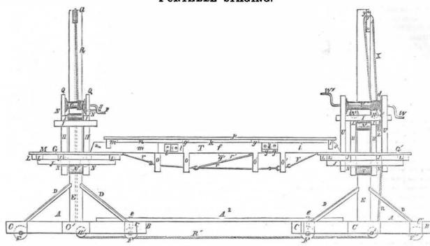
workmen to walk on. In using this staging | turning either or both of the cranks, W and | , ang s gised by farmers for therin fruit; it or lower it by turning the crank, P, and the tinue the bridge, T, in a horizontal position. workmen on the platform, G', can raise or lower both platforms at the same time by
