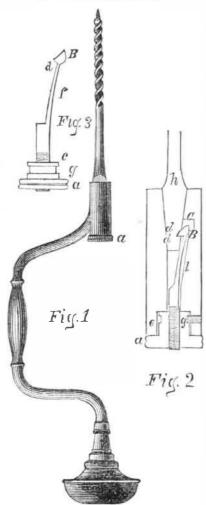
The annexed engravings represent an imroved mode of fastening auger and other bits to their sockets, for which a patent was granted to Ebenezer W. Nichols, of Worcester, Mass., on the 15th of May last. Fig. 1 is a side view of a bit stock, with an auger in it; fig. 2 is a half section of that part of the stock in which the shank of the auger or bit is fastened, and fig. 3 is a detached view of the burr nut and steel spring. Similar letters refer to like parts.
