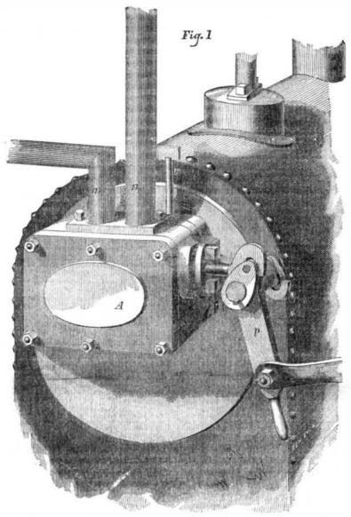
ratus for supplying steam boilers with water, for which a patent was granted to Benjamin F. Bee, on the first of August last, to which the rocking shaft, T, and lever, P, fig. 1. It is he has given the title of Hydrestant. Figs. 2 and 3 are sectional views of the apparatus, showing the internal arrangements and the different positions the two valves are made to occupy, by which contrivance water is
