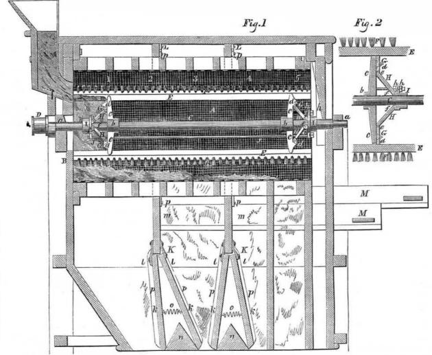
moving the slide to which the first division plate K, is attached the flour receptacle is enlarged or contracted so that only the first quality may be received in the flour receptacle. The same operation may be applied to the plate, K.
