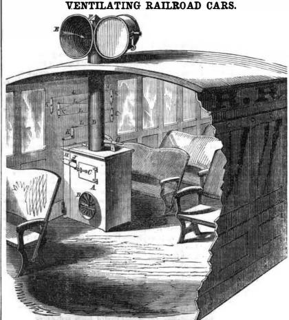
The accompanying engravings represent a | C, inside of it. F is the smoke pipe of this method of ventilating railroad cars, for stove, passing out at the roof of the car .which a patent was granted to B. T. Babbitt, of this city, on the 30th of January last.
