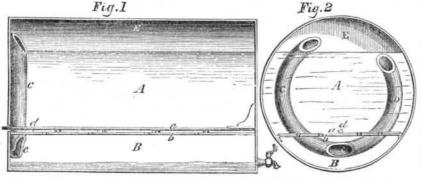
improvement in cleaning boilers, for which a with an opening, c, under the partition, b, patent was granted to Hiram Strait, of Covington, Ky., on the 4th inst., and his claim one end of this tube is open in the steam published in the Scientific American, in the space, the other is a little below it in the
