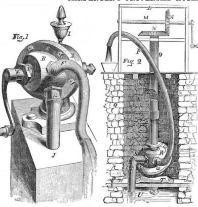
With a good breeze, it fills two tanks hold- our railroads it appears to be such a pump ing 24,000 gallons of water, in 2½ hours, and as is wanted. this water has to be raised 75 feet. It is a simple and strong pump, not easily injured, | ter addressed to Mr. Carpenter.
