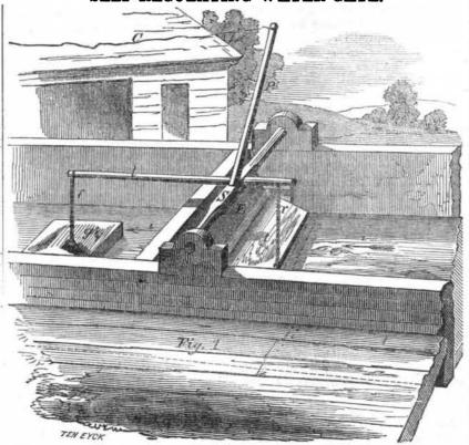
The accompanying figure is a perspective | clined position, which, in most cases, will be of Dundaff, Pa., on the 20th of February last. The arrows, 11, show the direction of the work. E represents a solid back of mason, or wood work built across the canal, and in or sluice, t. The back, E, is inclined out-
