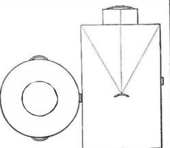
Length of case, 14 inches; diameter of case, 124 inches; length of cupola, 4 inches; diameter of cupola, 4 inches; length of tubs,  $\frac{3}{4}$  inches; diameter of tubs. 11 inches.
