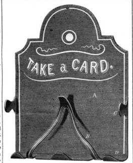
the case is struck out; so also are the small lugs or guides, C, at the side, and the bottom, D, which the cards rest upon. In this arrangement of the several parts, and the general details, a neat and convenient receptacle for business cards is furnished which can be sold at a low price, and will answer the purpose admirably.
