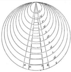
readers will understand the diagram without any explanation from us. The lines from a to a, represent the depth of the key-seat for wrought iron which in the largest size shown in the diagram is 1/2 inch in depth for 11 inches in width for wrought iron, and God 19 by 11 for cast-iron. These latter sizes are back, and is now sailing on the salt.
