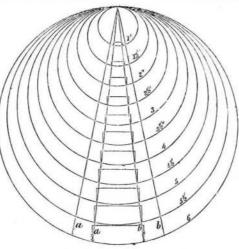
readers will understand the diagram without any explanation from us. The lines from a to a, represent the depth of the key-seat for wrought iron which in the largest size shown in the diagram is  $\frac{1}{2}$  inch in depth for 11 inches in width for wrought iron, and God  $\frac{9}{16}$  by  $1\frac{1}{4}$  for cast-iron. These latter sizes are back, and is now sailing on the salt.
