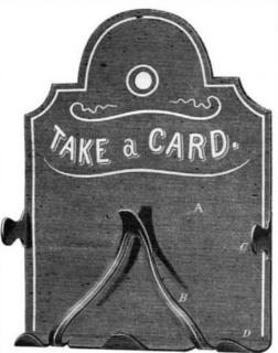
the case is struck out; so also are the small lugs or guides, C, at the side, and the bottom, D, which the cards rest upon. In this arrangement of the several parts, and the general details, a neat and convenient receptacle for business cards is furnished which can be sold at a low price, and will answer the purpose admirably.
