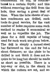
cured by a small key at the back. The shape of the cutter fitted in the key-way, of course varies with the work to be done, and the corners may be rounded
