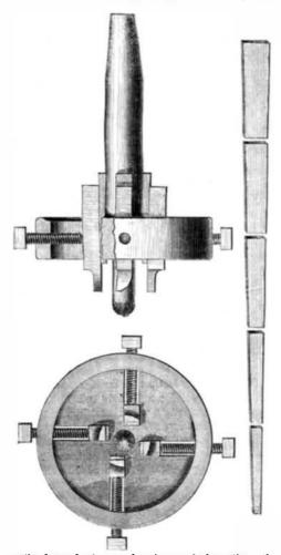
easily dressed when broken in much less time than the counter-borer could, thus making it cheaper to use both in point of execution and cost of repair when injured. We are indebted to Mr. Herman Winers, an accomplished engineer, now with Donald McKay, Esq., of Boston, Mass., for the plan of the tool presented above. It is, as may be seen, adinstable, and will cut holes of varying diameters, ac- up to it by inserting the center in the dead center of ary last, \$44,600.
