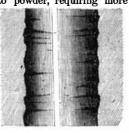
than Fig. 1; the edges are sloped directly from the cutting edge to the back of the drill and the point is thick and square. With such a drill as this a hole like this one, at the left, would be made, and for these reasons: the thick
