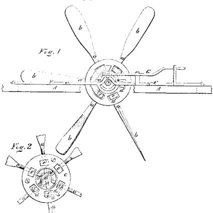
On the 6th of last June, a patent was granted to Thomas and Samuel Champion, of the City of Washington, D. C., for an improvement in the construction of paddle wheels, represented in the accompanying engravings, of which fig. 1 is an elevation of the paddle the wheel, showing the construction of the shanks of the paddles, whereby they are arranged in the same transverse line and passed through the hub. Similar letters on both figures refer to like parts.
