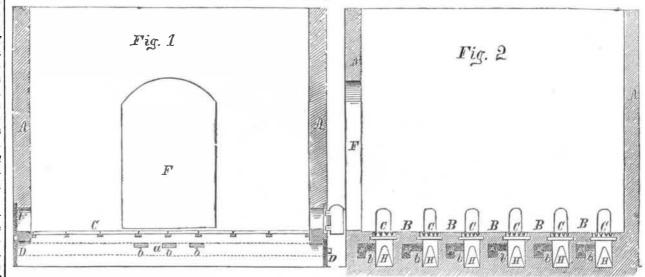
for the improvement in Brick Kilns, represented in these engravings, fig. 1 being a longitudinal vertical section, and fig. 2 a transverse vertical section of the kiln. This is a coal-burning kiln, and the improvement consists in a certain arrangement of the fire grates, and air passages, whereby very perfect combustion of the fuel is obtained, and regulated at all parts of the kiln.
