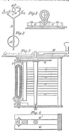
The hooks, e e', are furnished with projections extending beyond the wheel, and bent down, which strike against screws, g g', whenever the motion of the arm, by coming in contact with the set-screws, h h', has arrived on its extreme point. By these means, the progress of the wheel beyond the required distance is prevented:
