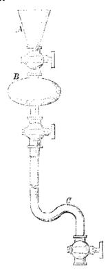
through the funnel on the top, and the upper cock is closed. By opening the stop-cock at the lower end of liquor. This might well be done to all the hydrants, the tube the mercury escapes into a vessel placed underneath, a column of 30 inches remaining in the tube; and a complete vacuum is obtained in the egg-shaped vessel, forming in this case the vacuum of Toricelli.
