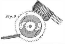
to those represented in Fig. 3, and the straps passing over the pulleys, e e, are fastened to the platforms, i i, which rest on rollers upon the inclined planes, rr; there being one of these platforms and straps, of course, for each foot, and the platforms having a reciprocating moshaft, are passed over the pulleys and fastened to the tion up and down the inclined planes as they are drawn cane pulp and 25 per cent. of rags
