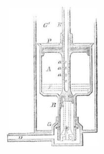
fills the upper part of the cylinder, and the small one the lower part. Near the lower end of the small part of the cylinder are other holes, o o, in the cylinder itself, which holes are within the iron water-chamber, G.
