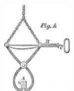
$\Lambda$ , is a section of the tire or other iron grasped by the hook. The tube, B, is firmly fastened to one arm of the hook and the rod, C, to the other arm. A workman, by taking hold of the tube, B, with one hand and of the rod, C, with the other, is able to open and shut the hook while standing at a tolerable distance from the fire. By having two or three of these hooks attached to the crane, the tire may be quickly and easily raised from the furnace although bedded in coal.
