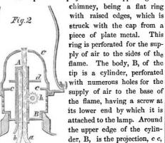
being an annular plate. Above this projection is the disk, d, fastened to the wick tube. The object of these
