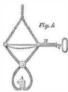
A, is a section of the tire or other iron grasped by the hook. The tube, B, is firmly fastened to one arm of the hook and the rod, C, to the other arm. A workman, by taking hold of the tube, B, with one hand and of the rod, C, with the other, is able to open and shut the hook while standing at a tolerable distance from the fire. By having two or three of these hooks attached to the crane, the tire may be quickly and easily raised from the furnace although bedded in coal.
