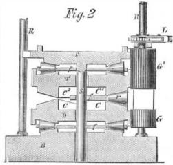
When the press is used as a punch, the punch is attached to the lower end of the shaft, S, the follower is braced in its place, and the upper disk only caused to revolve by means of a crank attached to one of the friction rollers which interpose between it and the follower; the gears, G and G2, in this case being dispensed with.
