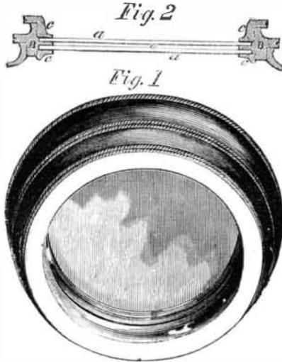
In the annexed engraving, Fig. 1 represents a perspective view of the whole, and Fig. 2 the several parts. B B, is the common bezel, a a, the plates, e, the space that separates them, and c c, the screws by which they are pressed firmly to their beds. They are packed water-tight by rings of india-rubber cloth, and a ring of india-rubber cloth is interposed between them at the edge.
