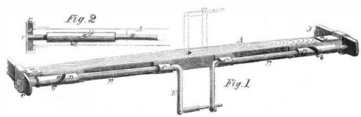
A a whiffle-tree detached from the axle-tree of a carriage. BB, are two rods which are fixed in the back of A, by guards, C, and D, and they are capable of longitudinal motion in opposite directions by means of arms or cranks. E.E. which are bent portious of the rods, and are operated by the driver by means of a chain or rope. The guards, D, have slots, a, made in them obliquely to the axis of the rods, B B, by which the cranks E, be-
