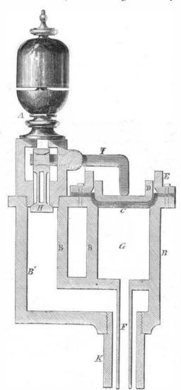
a valve, through which the steam can pass, and call attention to the state of the water in the boiler by a whistle. Our engraving, which is a section, will explain the construction.
