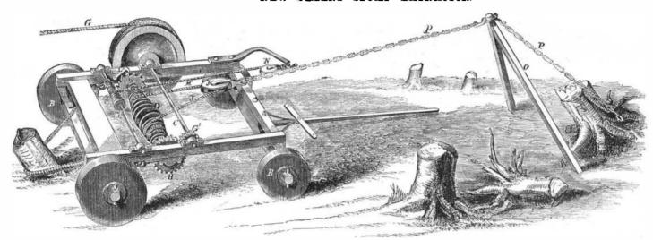
the outer side of the frame, which receives a rope or chain, G, to which the animal is attached to operate the ma-On the other end of the shaft a pinion, G', is placed that gears into a wheel, H, on D; H also gears into a pinion on E.
